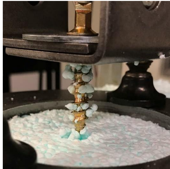
Figure 8. Pull-out test results for the 50mm thick EPS type II foam core (sample #5) under 3.125” diameter circular boundary condition.
