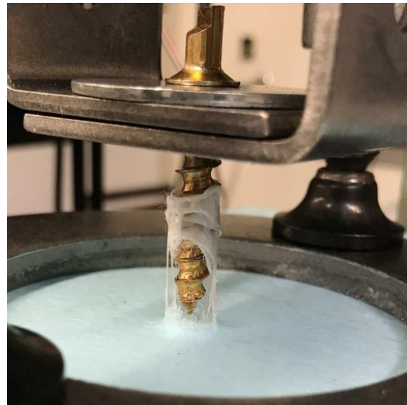
Figure 9. Pull-out test results for the 20mm thick Honeycomb core (sample #6) under 3.125” diameter circular boundary condition.
