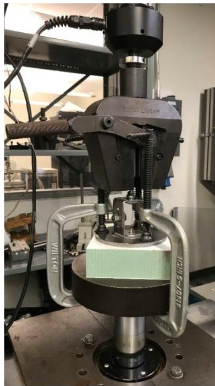
Figure 1: Pull-out test setup with the 3.125" diameter circular boundary condition.
