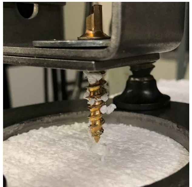
Figure 6. Pull-out test results for the 50mm thick PET foam core (sample #3) under 3.125” diameter circular boundary condition.
